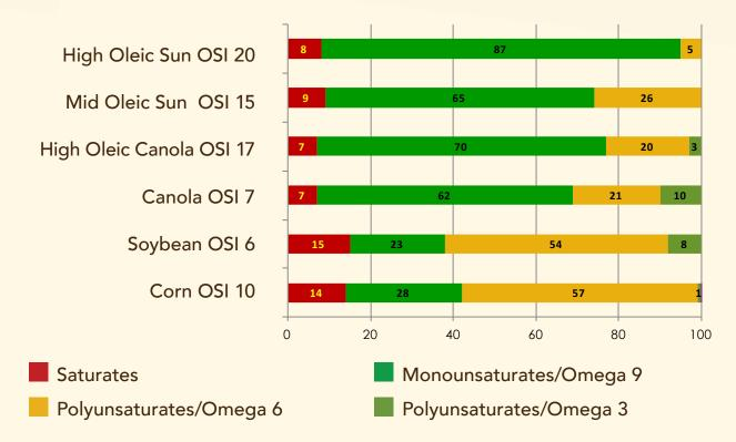
OSI measures the length of time (in hours) before a rapid acceleration of oxidation occurs (i.e. High Oleic Sunflower Oil will last 20 hrs vs. High Oleic Canola will last 17 hrs)
